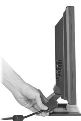
4. Connect the other end of signal cable to the signal connector of your computer.
